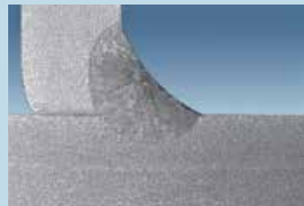
WIG DC, VARIGON® H6, v_s = 18 \text{ cm/min}
