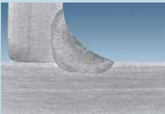
WIG DC, Argon, v_s = 13 \text{ cm/min}
